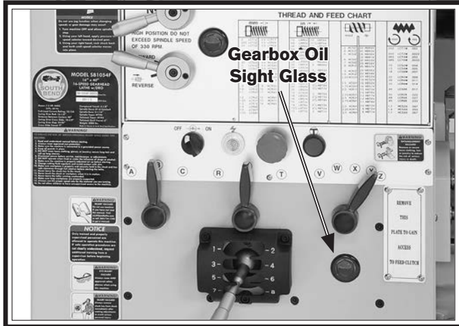
Figure 108. Location of quick-change gearbox oil sight glass.
